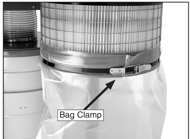
Figure 30. Canister filter collection bag installed.
